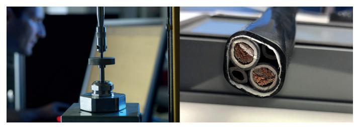
In order to enable customers to compare products, a cable-like test mandrel was defined by IEC / EN 62444 and required to have certain characteristics. The hardness of the test mandrel must be 65 Shore D  $\pm$  15 and the surface roughness Ra may not exceed 7  $\mu$ m. This ensures that all cable glands are tested identically.
