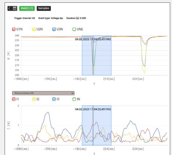
PQ event recording of a PQ5000MOBCLM with zoom option
