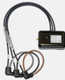
Current Module 3P, with 3-fold Rogowski converter
